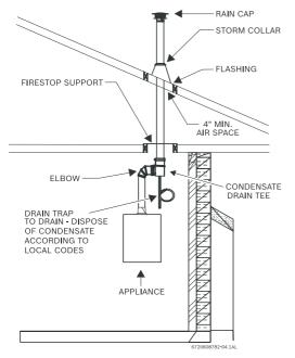
Fig. 15 Condensate drain installation
